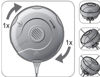
**b.** Turn the top portion one click clockwise to the next stop. Keep the Membrane Changer horizontal! Hold the changer's bottom half in place while turning the top half.
