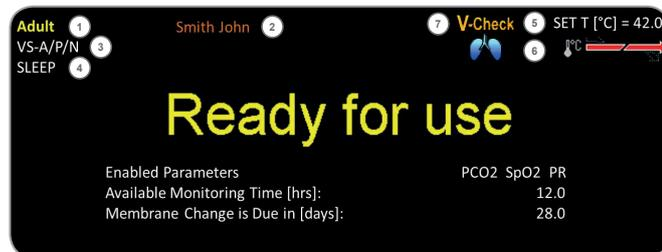
**Note:** Pressing the Enter Button (p. 42) while the 'Ready for use' screen displays activates a 'Quick Access Menu' with the possibility to activate additional calibrations (p. 16), to access the sub-menu 'Profiles', or to activate the V-Check™ Mode (p. 35).
