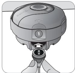
**2.** Place the Membrane Changer on a horizontal, dry surface with the colored dot facing up.
