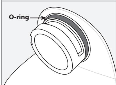
Visually inspect O-rings on nebulizer cap for cracks and damage.
