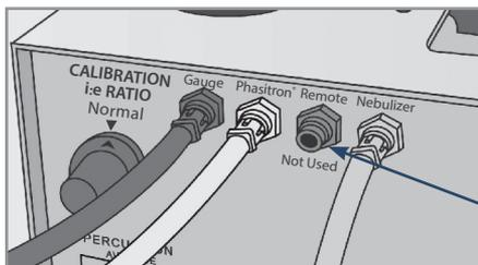
Connect red, clear, and yellow tubing connectors to the Impulsator® Model F00012 controller device.
