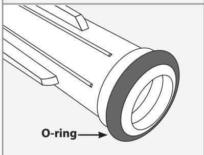
Visually inspect O-rings on sliding venturi for cracks and damage.
