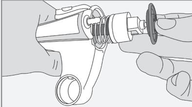
Insert venturi and spring into Phasitron® 5 body.
