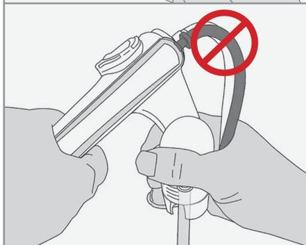
**⚠ CAUTION:** Do not bend nebulizer bowl while holding the tubing. This may cause undue stress on the red line conical connector.
