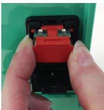
Replace red fuse carrier into the fuse panel by squeezing fuses together from sides and sliding fuse holder into housing.
