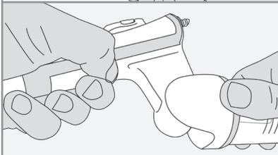
Add mouthpiece, mask, and corrugated tubing to the Phasitron® 5 as needed.
