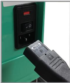
Plug the female end of the power cord into the back of the controller. Plug the male end of the power cord into a wall outlet.
