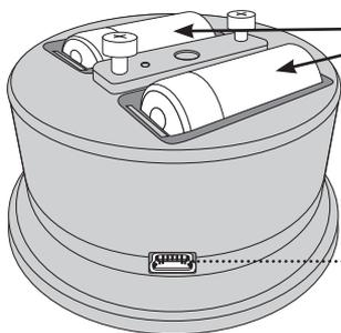
Install batteries into PDM
