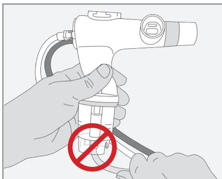
**⚠ CAUTION:** Ensure yellow nebulizer tubing is not bent. This may cause undue stress on connector.
