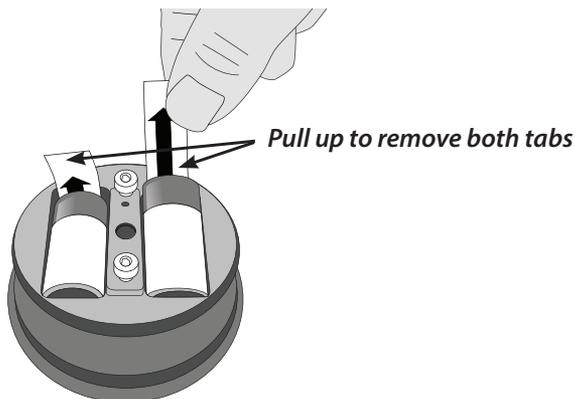
**NOTE:** To ensure correct atmospheric pressure calibration at start up, remove batteries, wait 30 seconds and reinstall. Allow 15 seconds for power-on self-test. When screen goes blank, the multimeter can be installed into the device.
