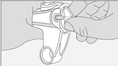
Screw white cap onto rear of the Phasitron® 5 body until stop.
