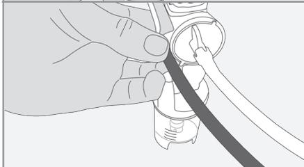
Connect the clear tubing quick-connect fitting to the cap at the rear of the Phasitron® 5 body.
