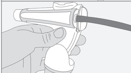
Press red tubing onto conical connector at rear of Phasitron® 5 body.
