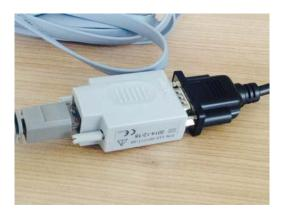
5. Use the Mindray type C serial port adapting cable (black cable) to connect the ID-Adapter with the female RS-232 connector on the rear of the SDM.
